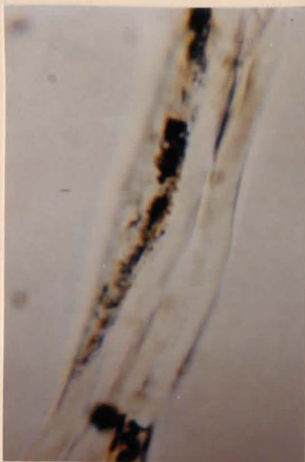
Figure 10 (left) sample 6BF after 2½ months in Cargille oil. The red particles have turned black and a yellow substance is exuding from the particles. 650x by Kohlbeck.
