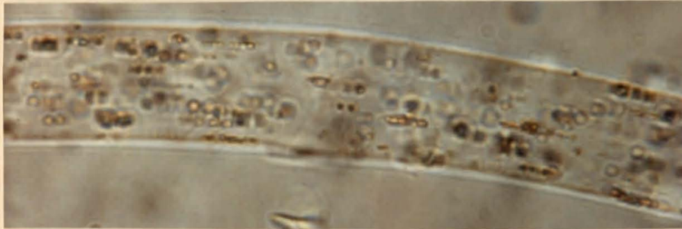
Figure 14, sample 3EF from the wrist wound area showing yellow and colorless particles on a fiber. 650x by Kohlbeck.
