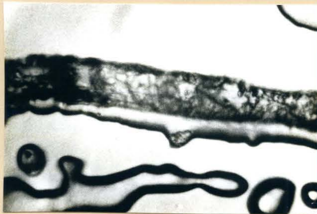
Figure 48, Detail of corroded fiber. Photographed at 400x by Damian.
