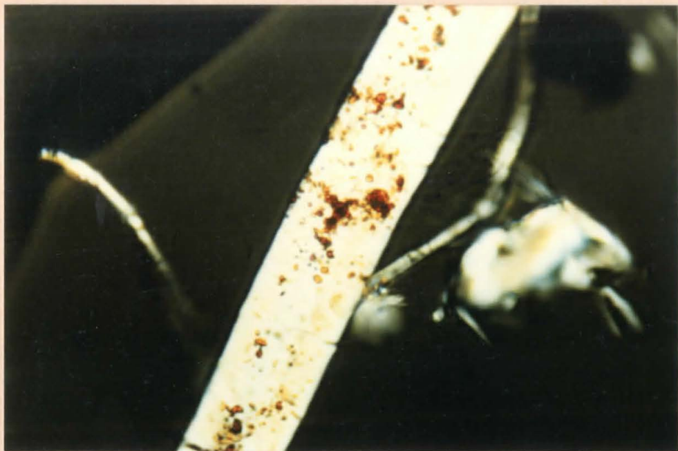
Figure 9, sample 6BF from the lance wound area. Red particles on Mylar tape before being remounted in Cargille oil. 650x by Kohlbeck.
